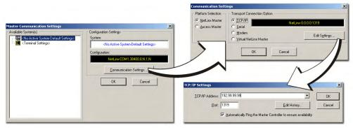
FIG. 28 Assigning Communication Settings and TCP/IP Settings
